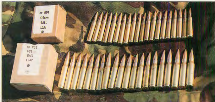
Below: The SA80's 5.56-mm ammunition is compared to the 7.62-mm rounds fired by the SLR. The SA80's lighter bullets are more affected by the wind, and you must adjust your aim to compensate. On the other hand, its lightness allows far more ammunition to be carried comfortably.
